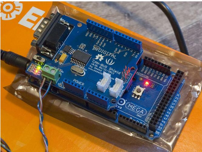
Take the twisted-pair cable and insert the bare end of the Grey/Red wire in the CANH port of the CAN-BUS shield. Insert the bare end of the Blue/Red wire in the CANL port. Secure the wires with the port screws.
