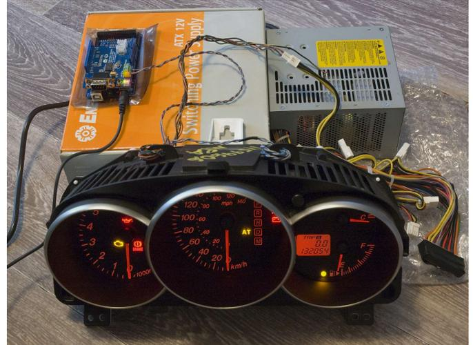
Now turn on the power supply and verify that the cluster is doing its starting routine. The needles should go all the way up and then down.
