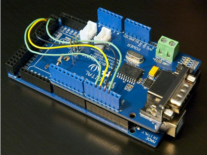
Install the CAN-Bus shield on top of the Arduino Mega board.
