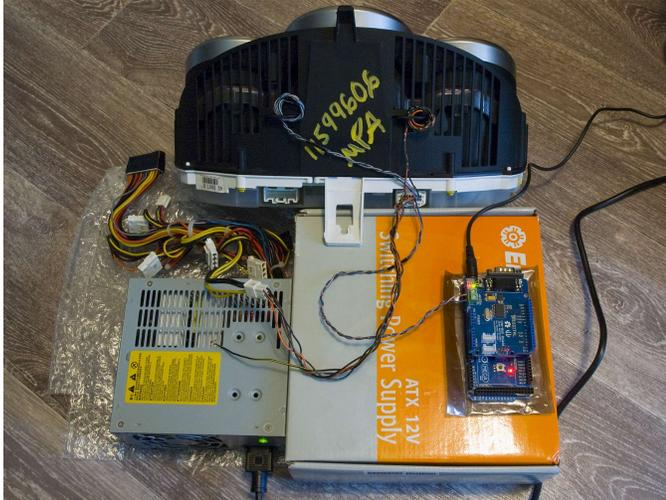
The final configuration should look like in the picture above once all the wires and components are connected. At this stage you can connect the Arduino board to a USB port of the PC and to a wall outlet using the AC/DC 12 volt power adapter.
