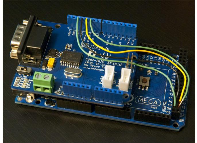
Create a special bridge between the CAN-BUS shield and the Arduino by connecting the 4 wires in the following sequence:
