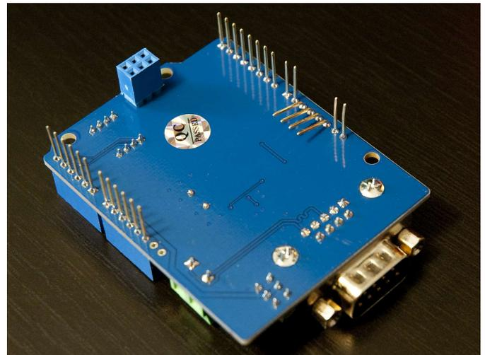
Take the CAN-BUS shield and place it upside-down. Locate the 4 pins numbered 10-11-12-13 and bend them delicately with tweezers like depicted in the picture above.
