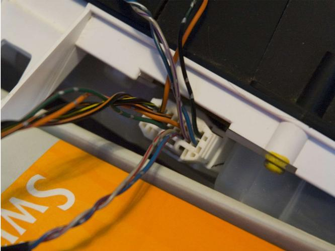
Pick the smaller cable harness, seat it in the proper port of the instrument cluster and isolate the four following wires:
