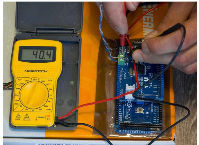
The resistance on the CAN-BUS shield CANH and CANL ports should indicate 40 Omhs.
