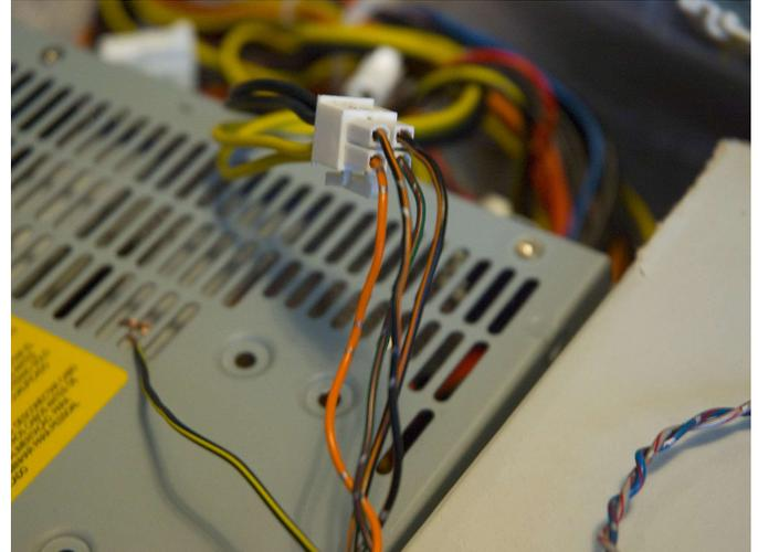
Take the 12 volt connector of the power supply and identify the two black-wired ports and the two yellow-wired ports.
