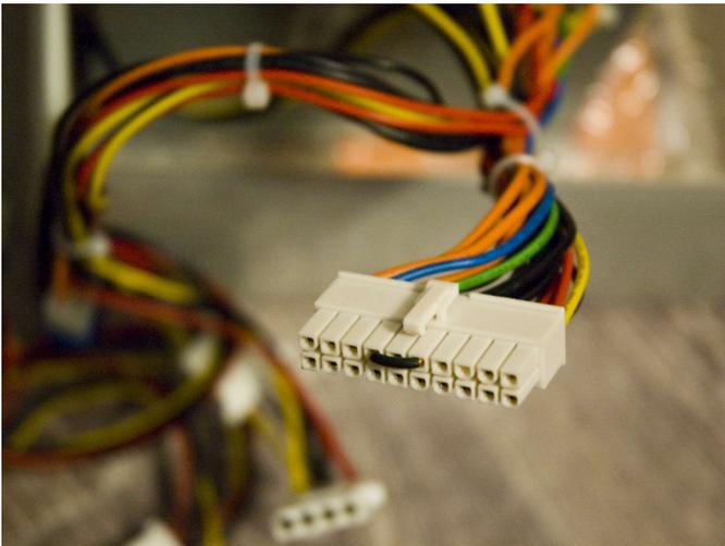
Take the 20-pin connector of the power supply and jump-connect the green and black-wired ports in order to start the power supply as soon as it's connected to a AC wall plug.
