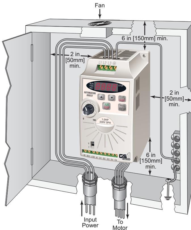
**MAXIMUM AMBIENT TEMPERATURES MUST NOT EXCEED 40°C (104°F)!**
