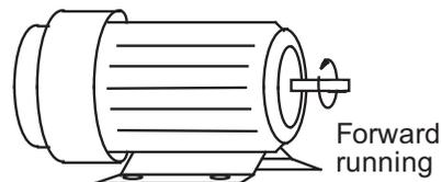
7. When the AC drive output terminals T1, T2, and T3 are connected to the motor terminals T1, T2, and T3, respectively, the motor will rotate counterclockwise (as viewed from the shaft end of the motor) when a forward operation command is received. To reverse the direction of motor rotation, switch the connections of any of the two motor leads.
