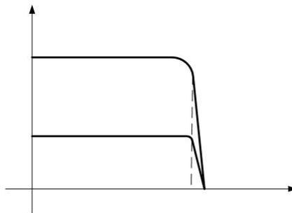
M<sub>max</sub> of LB and LBB series servo motor is equal to 3M<sub>n</sub>; M<sub>max</sub> output status is the short time work of the servo motor. Please refer to the output capacity of the matching driver before use.
