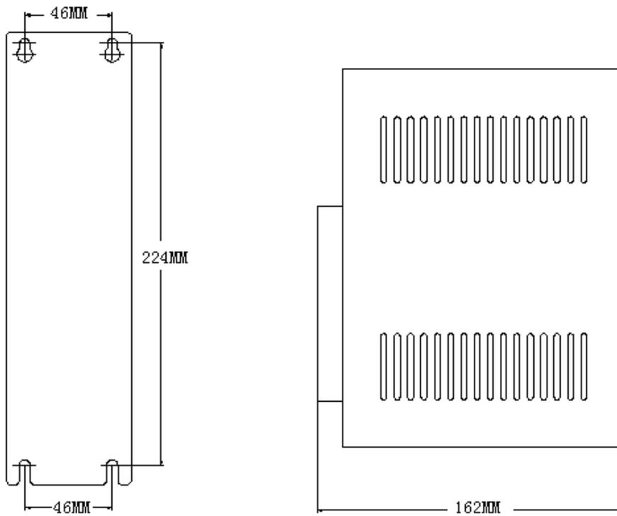
**Figure 1.11 Installation Dimensions
