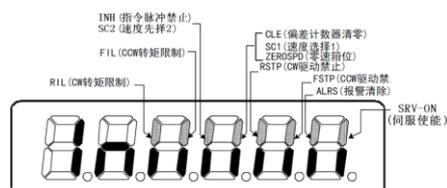
Figure 5.2 Display of Input Terminal Status
