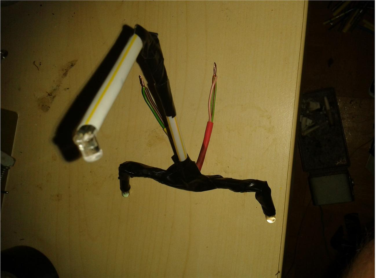
Now i solderd a cable with an 3,5 mm audio plug to the Model. Connection + wires to the top and – at the bottom. And mountet this on my headset.
