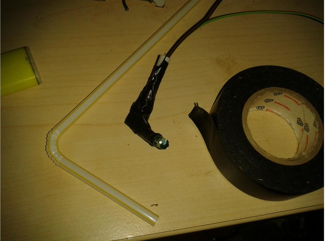
When you let the soldering ends of the Leds very long later it is easier to adjust them.
